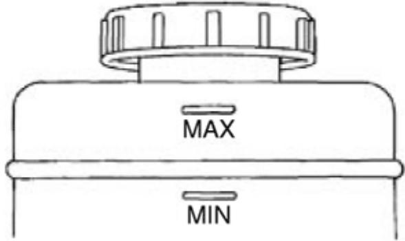
Use only hydraulic brake fluid conforming to DOT 3 or DOT 4 specification.
